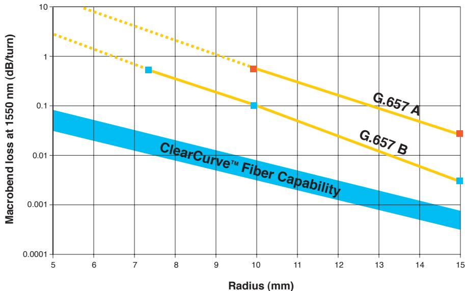
Figure 4. Extrapolation of ITU-T Recommendation G.657 performance to 5 mm and comparison with Corning's ClearCurve optical fiber.
