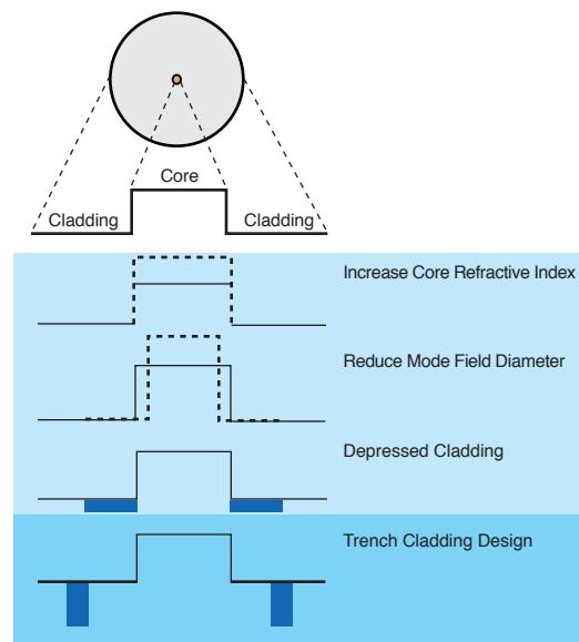
Figure 2. Alternative designs for improved macrobending performance to meet requirements of Recommendation G.657.
