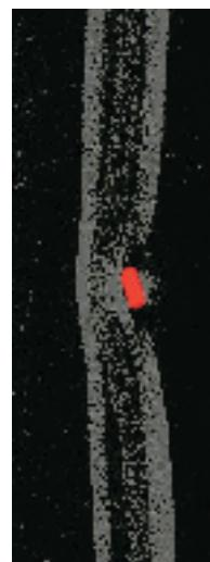
Figure 3. X-ray of bending of fiber in miniaturized cable due to direct affixing using stapling technique.
