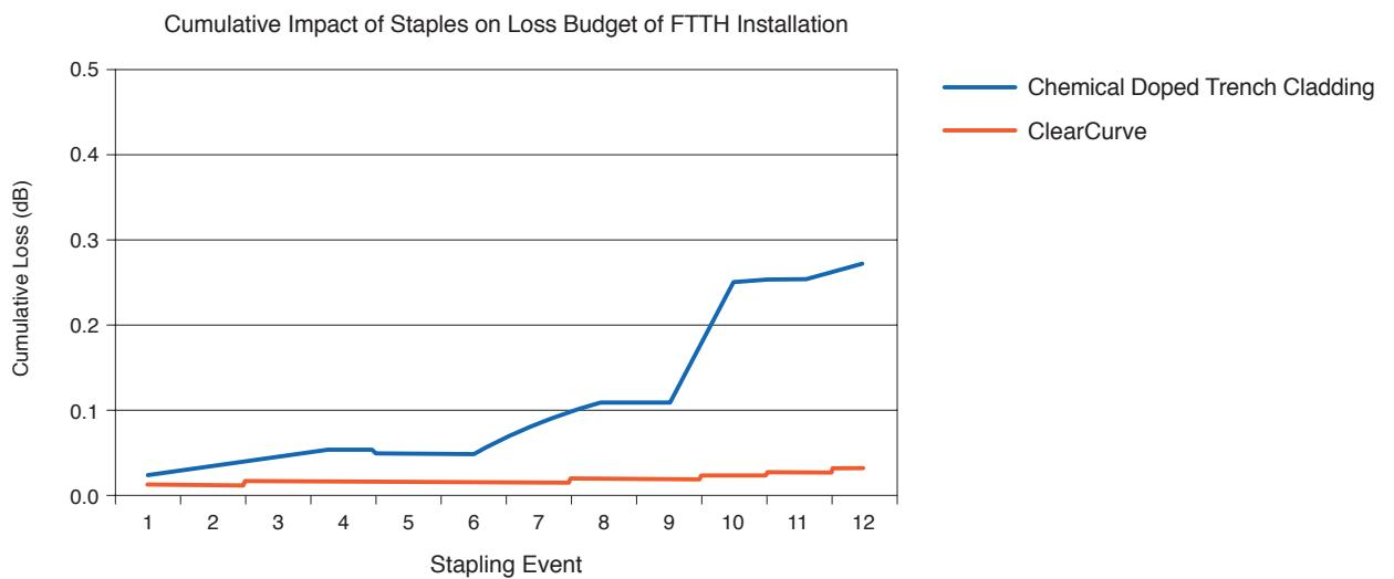
Figure 5. Comparison of bend loss due to incremental stapling in miniaturized cables.
